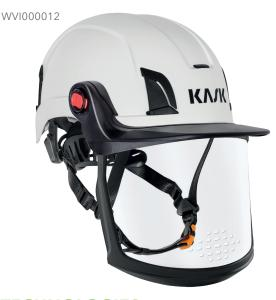
Ventilated polycarbonate face protection designed to work with all Zenith series helmets. EN 166 rated to protect the faces of workers from medium level energy impacts while enabling greater airflow and circulation. Available in 2 lens color options for various levels of light transmission. Securely flips up and down. Attaches with Easy Click Visor Adaptors and ZEN Face Shield Carrier.
